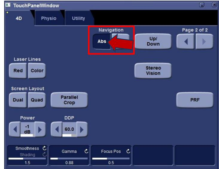
For 4V-D probe Abs is the default for factory presets
